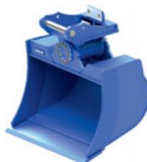
**HB 15 RM Universal tilting bucket****backhoe bucket shape with round side part**, 2 x 45° tilting range, with hydraulic tilt motor, base out of 400 HB steel, cutting edge 200x25mm out of Lehborit 5000 (500 HB)
