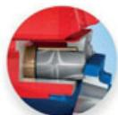
Quickcoupler incorrectly locked
