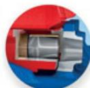
Quickcoupler correctly and completely in adapter, locking bolts still retracted
