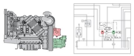
Picture 21: Base machine's pumps
