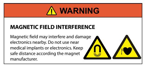
Magnet produces a strong magnetic field that interferes with electronic devices. Do not use electronic devices near the magnet.
