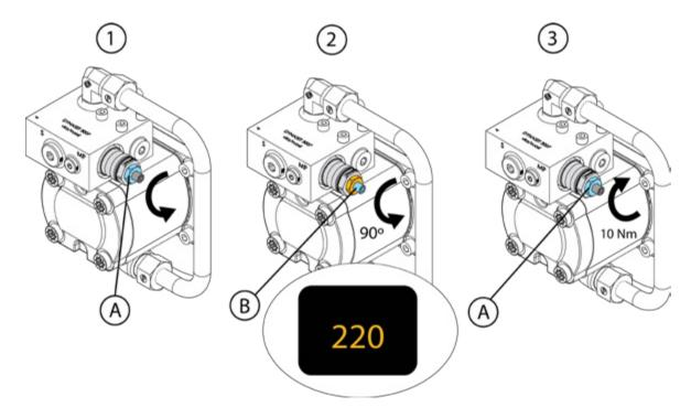
During the adjustment U.CUR will blink on the display. This is normal. Do not attach magnet on to the generator while measuring the voltage.
