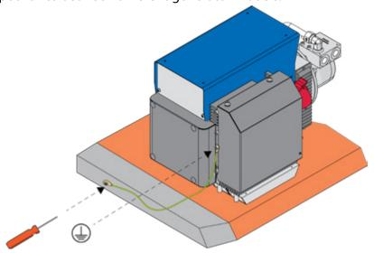
Picture 25: Grounding the HMG/CMG PRO hydraulic magnet generator
