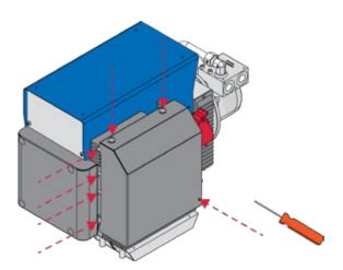
Picture 49: Installing the control box cover
