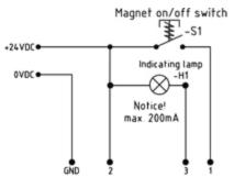
Control +24VDC (left valve plug)
