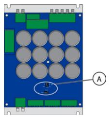
Picture 29: Location of the DIP switches on the control card
