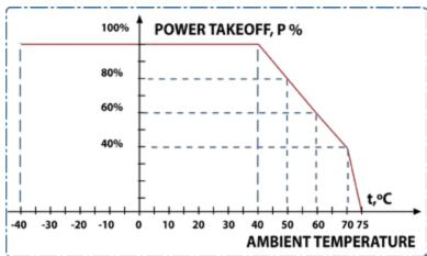
Picture 45: Power take off in higher temperatures
