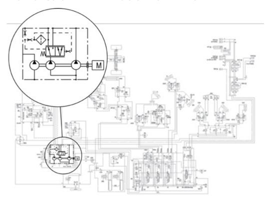
Picture 14: Open centre hydraulic system with constant displacement pump
