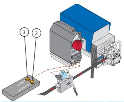
Picture 41: Operating the magnetization by controlling magnet generator's magnetizing voltage
