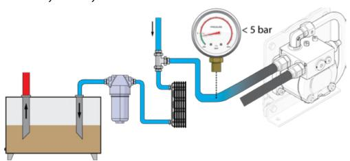
Picture 22: Return line (T) pressure must be under 5 bars.
