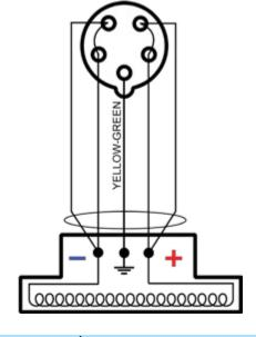
Picture 33: Wiring for the cable from the generator to the magnet
