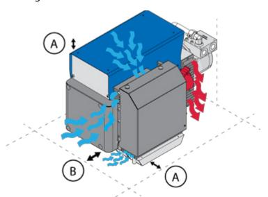
Picture 23: Placement of the HMG/CMG PRO hydraulic magnet generator.
