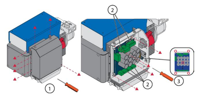
Picture 47: Removing control card
