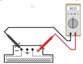
Picture 39: Measuring resistance from the magnet
