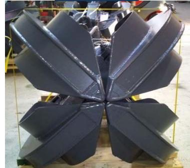
**Multi-jaw grab with 5 grab cylinders and rotary feed system**
