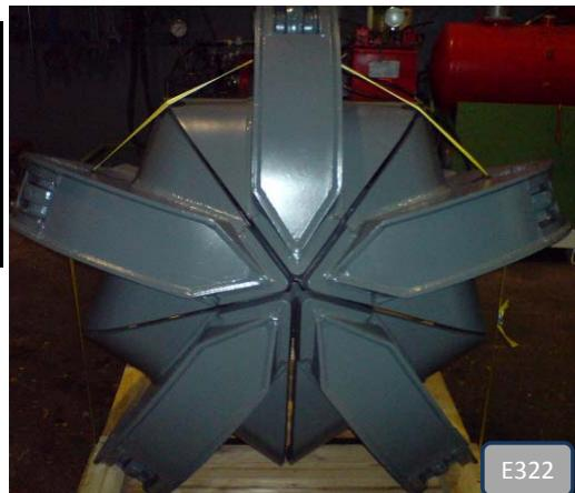
**Multi-jaw grab with 4 grab cylinders and rotary feed system**
