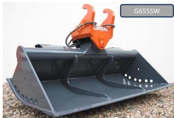
**Trench digger, bucket shape with rear blade and fixed or swivelling 2 x 50 degrees with rotator HKS Xtra Tilt 250, with hoses up to the articulated jib with water holes in the rear wall**
